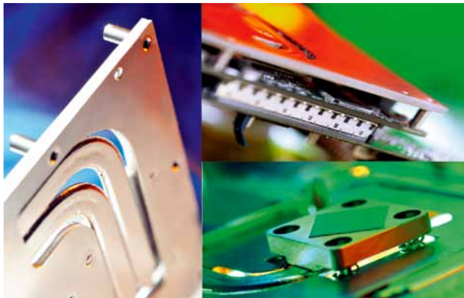
Congatecs värmeslits (heat pipe).
